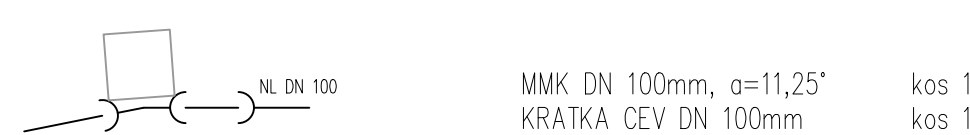
56 Horizontalni lomi 11,25°+11,25°+11,25°+9,25° in vertikalni lomi 16°+15°+0°+26°
